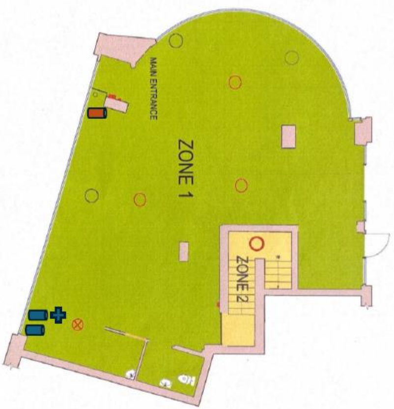
FIRE ALARM SYSTEM ZONE PLAN
