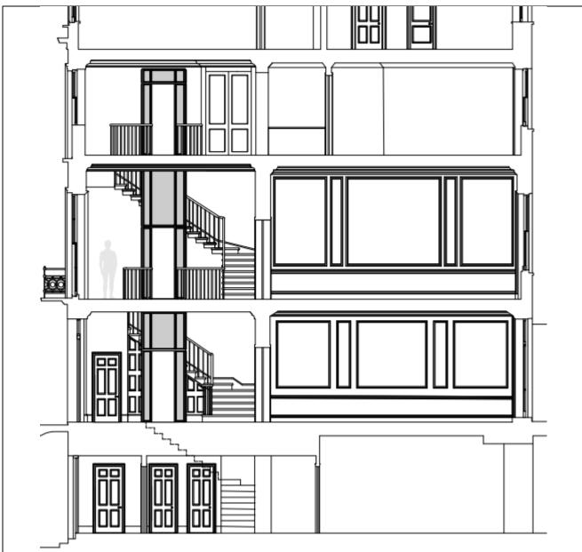
**Proposed section** through stairwell, showing new lift shaft, and breaks in balustrades at first floor and second floor.
